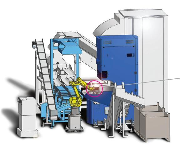
Presses with rotary table, hydraulic and/or electric
